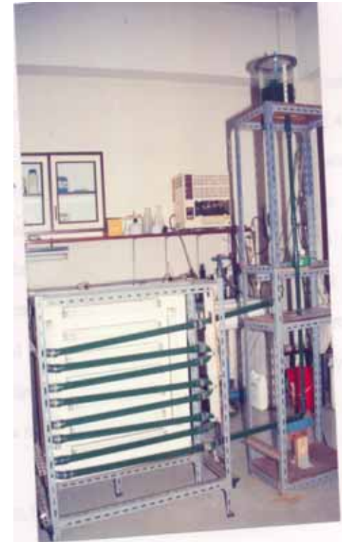
Glass tubular photobioreactor of 0.229 m 2 surface area, 3 cm diameter and 120 L working volume.
