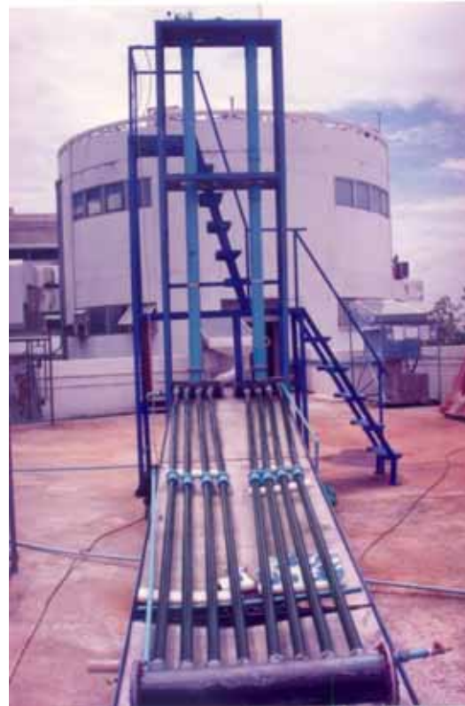
The outdoor tubular photobioreactor of 1.4 m 2 surface area, 4 cm diameter and 150 L working volume
