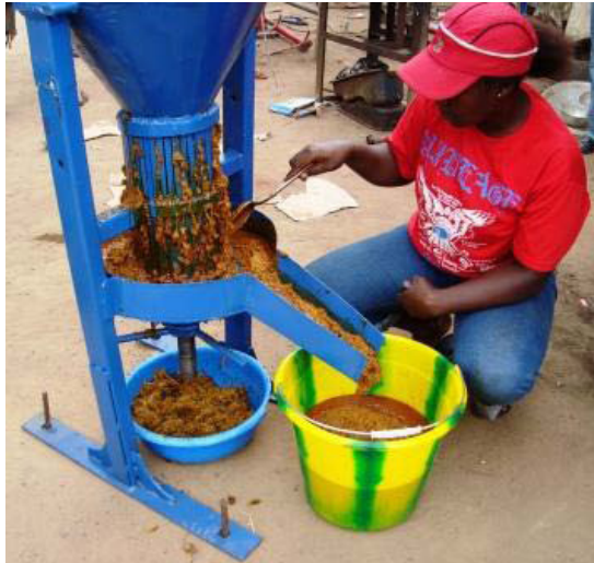
Figure 15 Mechanical processing with 'Freedom Mill'. Source: USAID, Winrock, STCP
